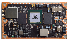
Figur 2.3: NVIDIA Jetson TX1 [18]
