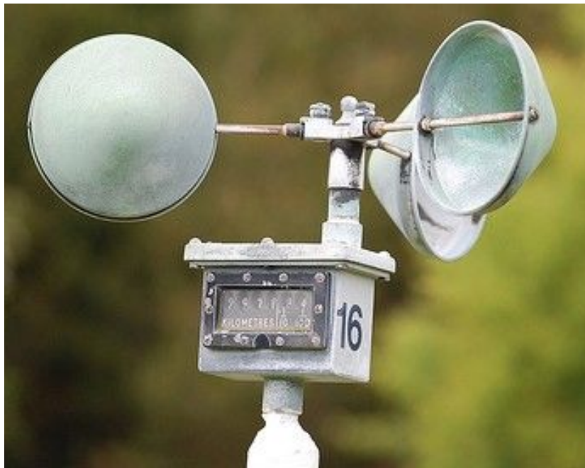
Figur 2.4. Kopp anemometer (Compact Analysis, 2016).
