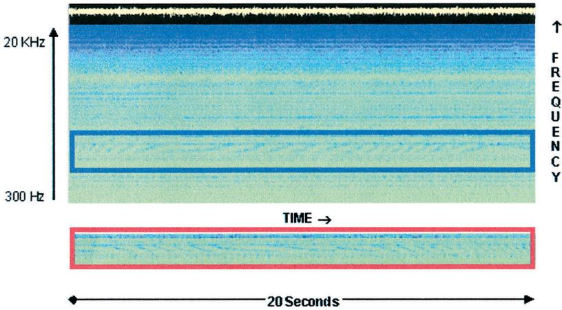
Fig. 12. Suspected Doppler signals with a gradually changing blue-shift (marked by rectangle) recorded by a VLF spectrometer. An example of gradually changing red-shift (marked by rectangle) is also shown below.
