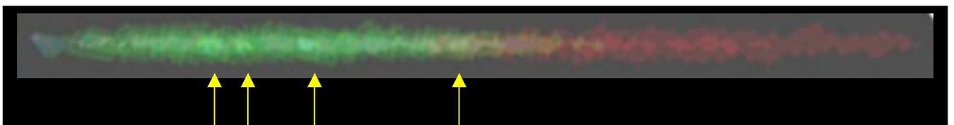
**Figure 21.** Low-dispersion spectra of the Hessdalen-lights of the blinking type. Date: August 21, 2001. Spectrum A (above) was obtained when the light was at maximum intensity: the corresponding 2-D color spectrum is presented with the most prominent emission lines marked (below). Spectrum B (middle) was obtained when the light was at intermediate intensity.
