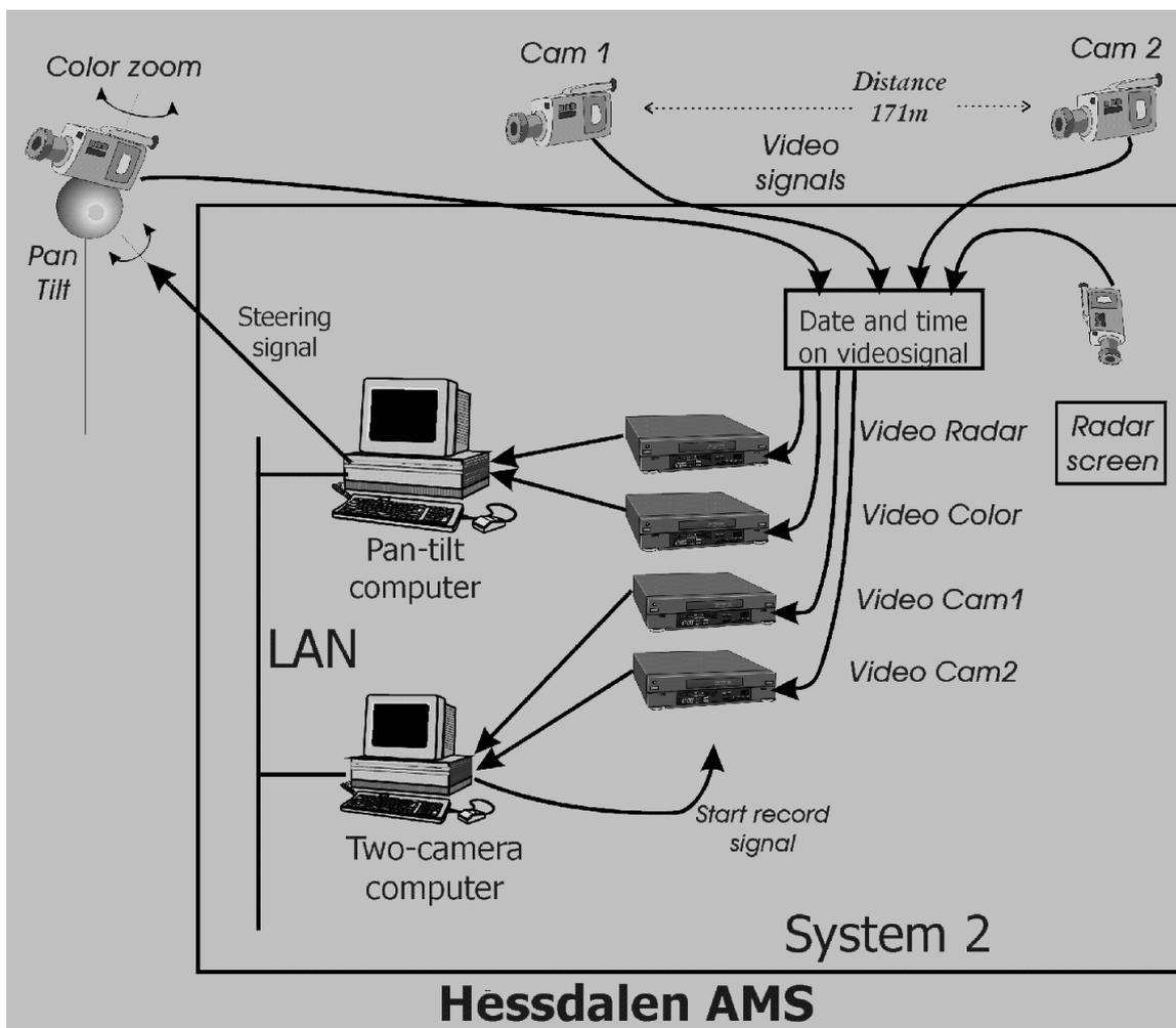
Figure 1. Flow-chart of the Automatic Measurement Station in Hessdalen (System 2).
